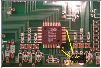
5) Double-check that the Driver pins are placed exactly over the pads. Now is the time to correct a misalignment by melting the tack solder, and twisting the part gently while the solder is liquid.
