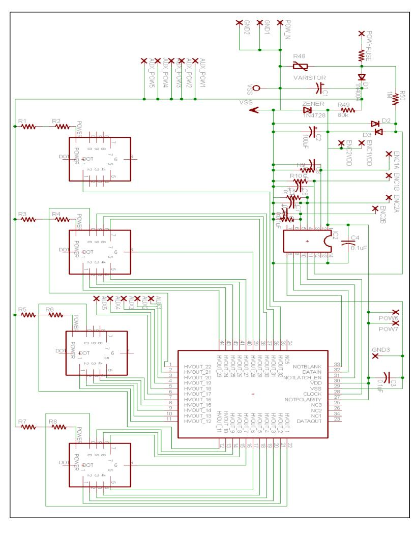
The low voltage supply is provided by a resistor and a Zener diode acting as a voltage divider. The <sup>1</sup>/<sub>2</sub> watt 82k Ohm resistor (R49) limits the current flow, and the Zener keeps the voltage at about 5V DC. A 100uF capacitor (C2) across the Zener filters the 5V power supply, keeping it stiff, and allowing the clock to go without power for 5 to 10 seconds without losing the time.
