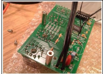
52)Slide the board into the enclosure front, sliding in from the right as you face the back of the clock. Slide the backplate on as you go. The leads from the buttons may need to be bent all the way out to clear the micro-controller as you slide in the back plate. (Alternative: you can bend the front panel wider open top-to-bottom, and snap the back panel straight in. Just be careful not to distort the front panel. This method works very well.) Note again that a 2-wire power cord is shown in the
