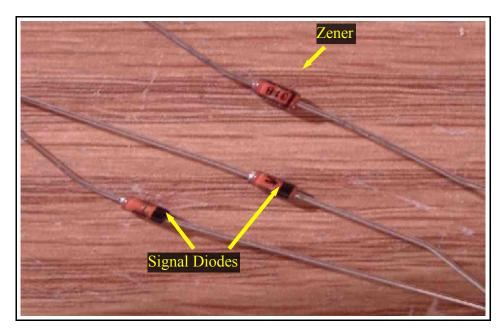
21)Solder the Zener diode, stripe towards the top of the board, in the place marked ZENER. MAKE SURE THE STIPE IS TOWARDS THE TOP OF THE
