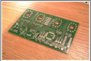
2) Locate the Driver surface mount chip, and place it on the PCB. Notice the orientation and pin alignment. The top of the chip goes to the right (the pin 1
