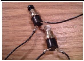
34)Slide a short piece of heat shrink over each wire and button lead, and shrink in place with heat gun or hair dryer. If a heat gun or hair dryer is not available, the heat shrink can be shrunk with careful use of the soldering iron, placed close
